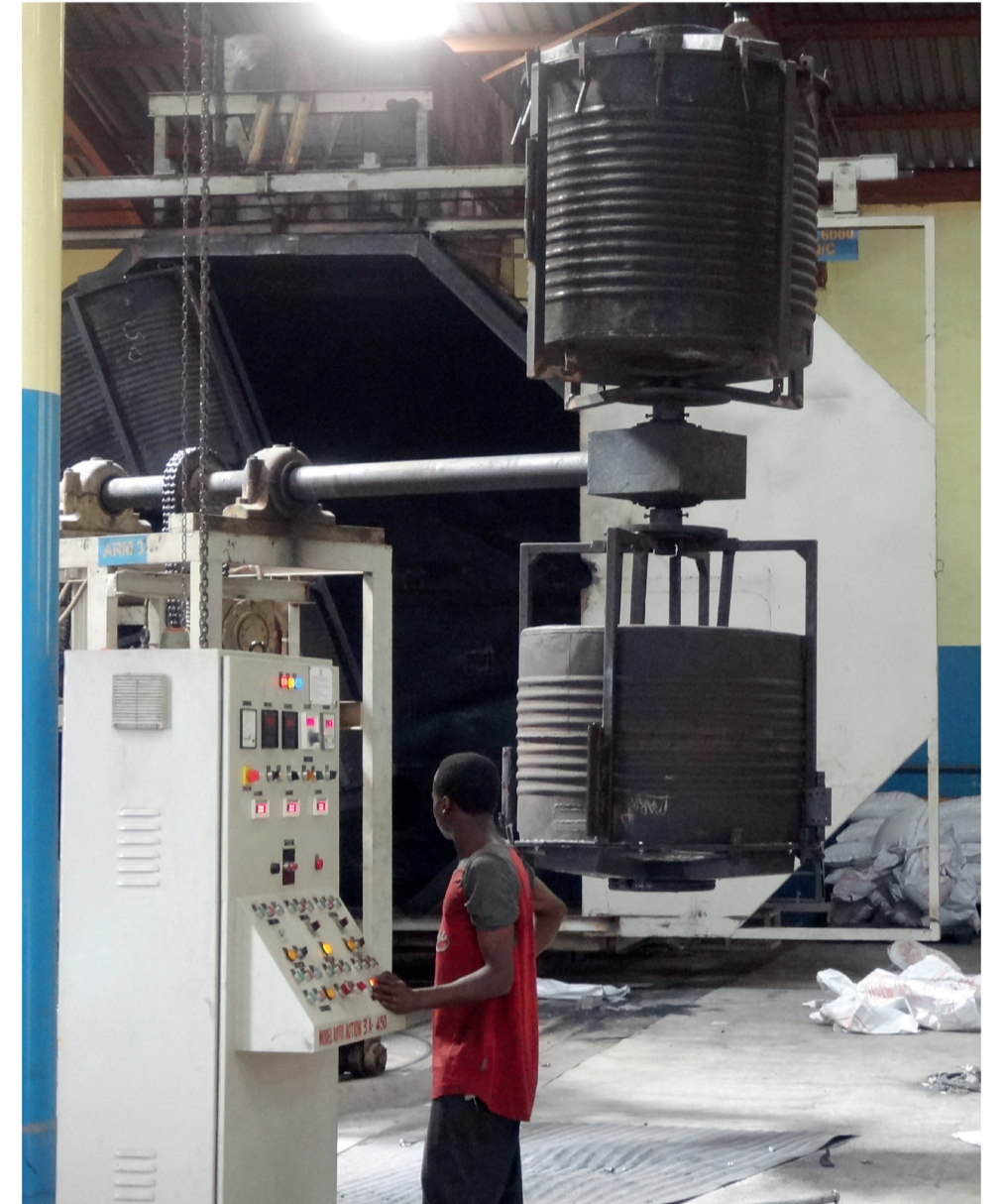
The water wall is produced by rotational moulding which is a widespread production technology.
